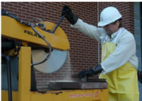
A worker cutting masonry block on a stationary masonry saw that continuously feeds water to the blade.
